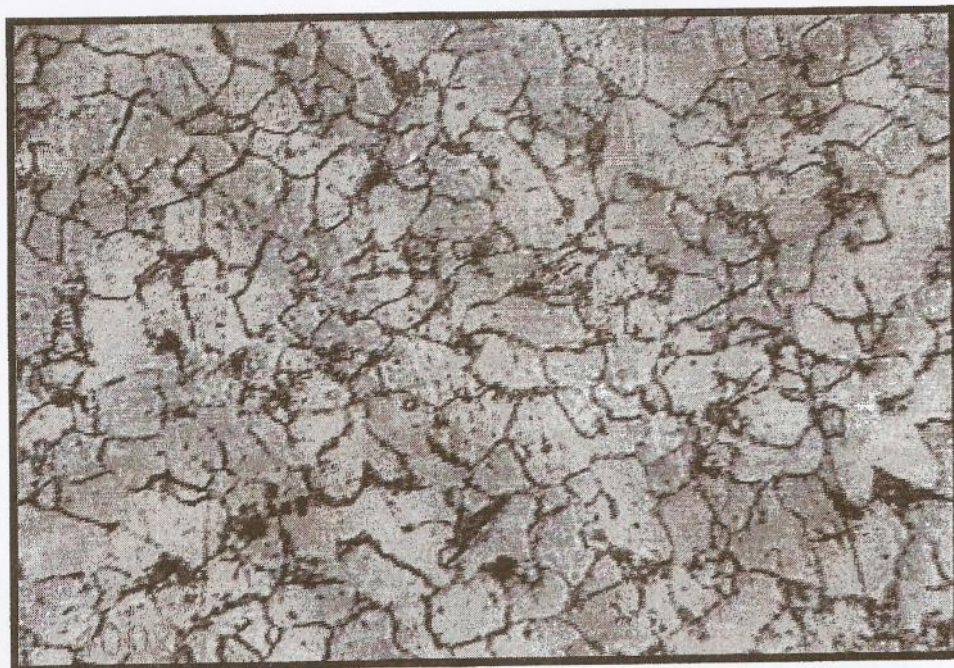
Plate 2- Distored microstructure of mild steel (106B ) showing the phase change ,specimen(2) ,etched by nital,400x.
