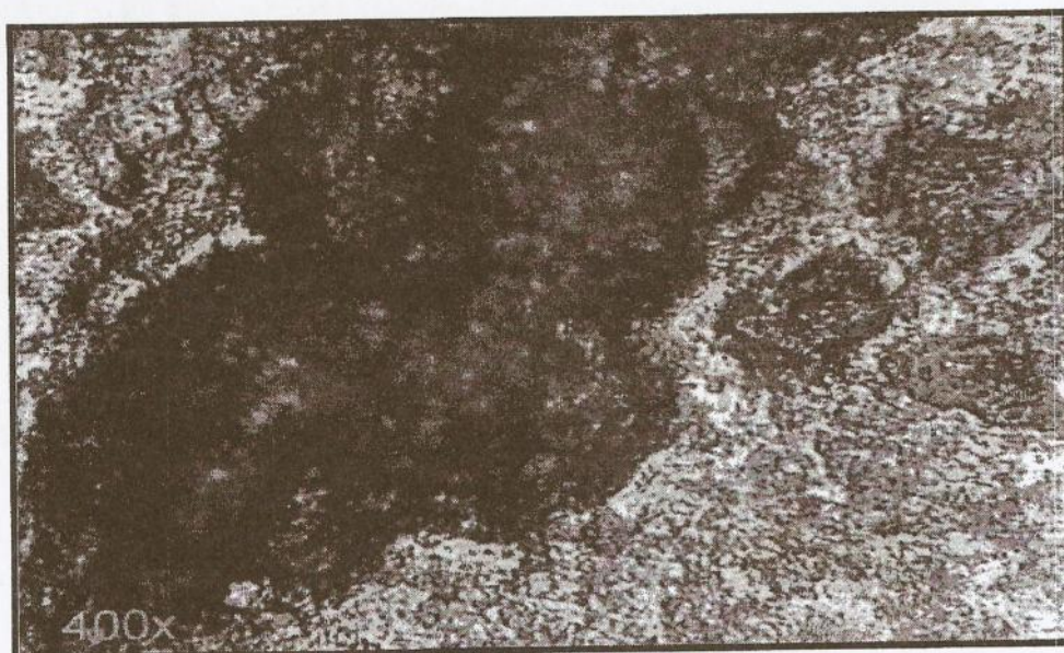
Plate 3- Surface feature of mild steel (106B) pipe interior showing the pitted areas, specimen (3) ,etched by nital,400x.
